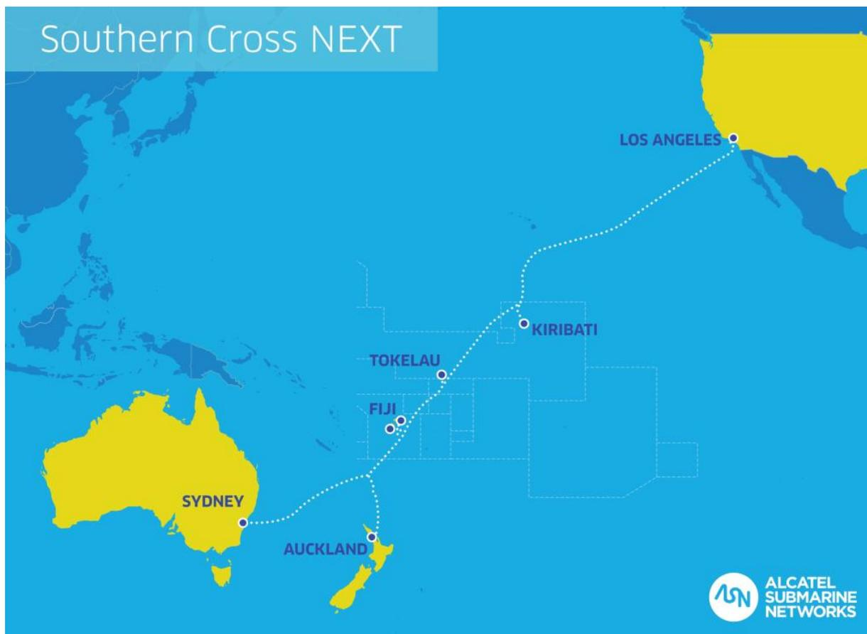
Southern Cross NEXT will connect Sydney and Auckland to Los Angeles providing the largest capacity and lowest latency connection between Sydney, Australia and Auckland, New Zealand to Los Angeles on the US West Coast. The system includes the latest generation of ASN repeaters, Branching Units (BU) and WSS ROADM, enabling additional branches to Fiji, Tokelau and Kiribati.
